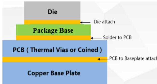
Figure5. Thermal Model Stack-up for DFN Package.
