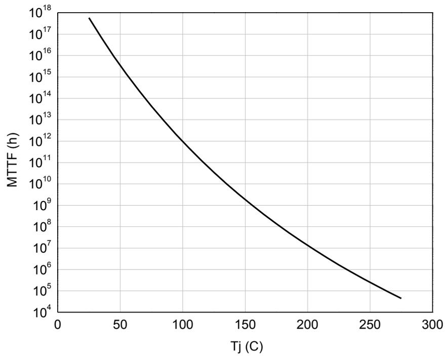
Fig 5. Median lifetime vs. channel temperature
