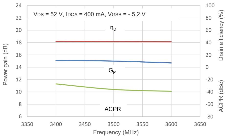
Fig 3. Single-Carrier WCDMA broadband performance @ Pout = 48.5 dBm Avg.
